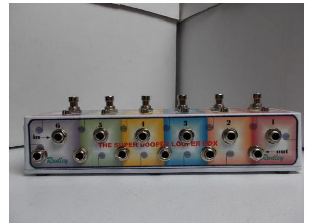
Back View – Inputs and Outputs to Pedal Effects.
